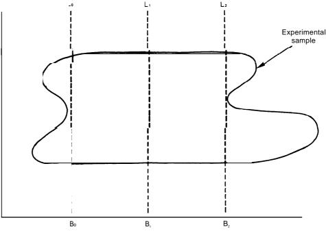
Figure A-3.—Experimental Sample in Magnetic Field Gradient
