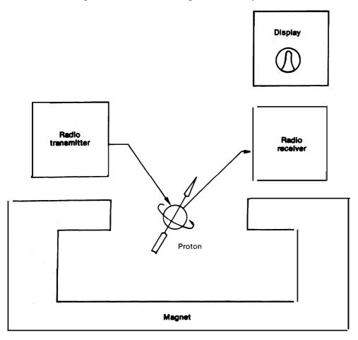
The radiotransmitter provides radiowaves at the appropriate rotational frequency to excite the proton. When the radiowaves are turned off, the excited protons precess in phase, thereby producing radiowaves that are detected with a radio receiver and then displayed.
