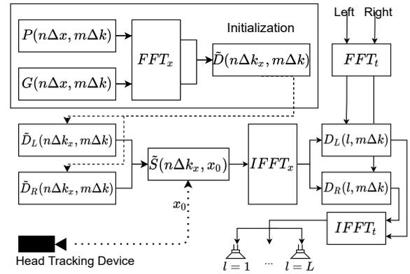
**Fig. 2:** Block diagram for the implementation. All quantities are represented in discrete form. The truncation and discretization processes are neglected.
