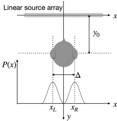
**Fig. 1:** Illustration of the specified target pressure distribution. Two spatial Hanning windows are centered at the positions of listener's ears ( $x_L, x_R$ ). The listener is located at  $[0, y_0, 0]^T$  as reference.
