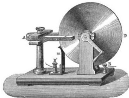
*The Faraday disk was the first electric generator. The horseshoe-shaped magnet (A) created a magnetic field through the disk (D). When the disk was turned, this induced an electric current radially outward from the center toward the rim. The current flowed out through the sliding spring contact m, through the external circuit, and back into the center of the disk through the axle.*
