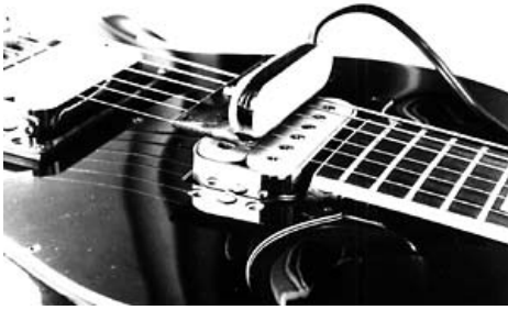
Fig.11. A transmitting coil radiates its magnetic AC field into the pickup coils. So you can measure the frequency response easily
