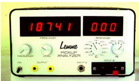
Fig.12. The "Pickup Analyzer" ® - the first commercially available measuring instrument for the frequency response of magnetic pickups.
