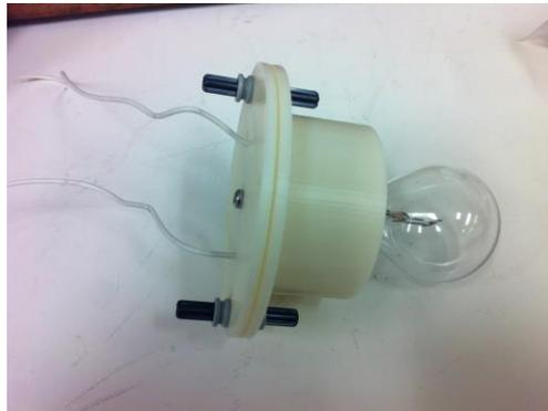
Figure 3 3D-printed Lamp Holder.
