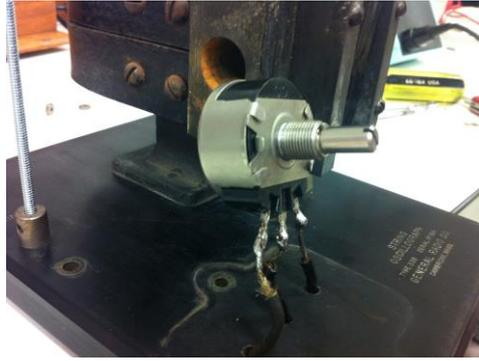
Figure 11 New Potentiometer.
