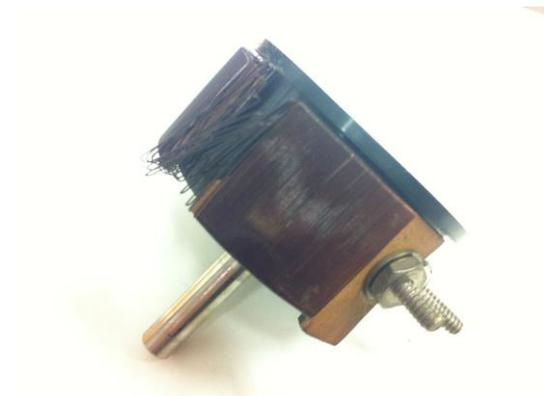
Figure 10 Broken Potentiometer.
