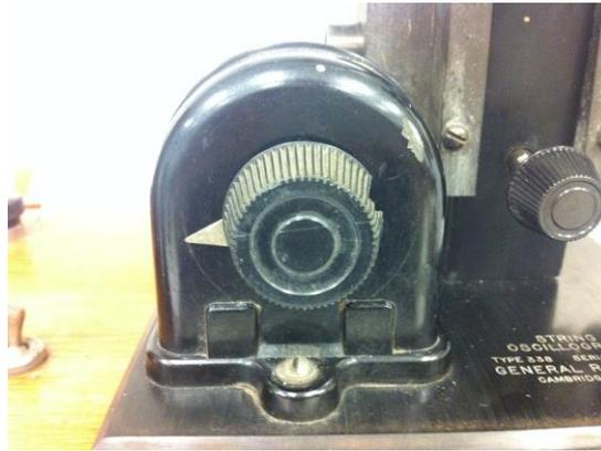
Figure 8 Adjustment Knob of the Potentiometer.
