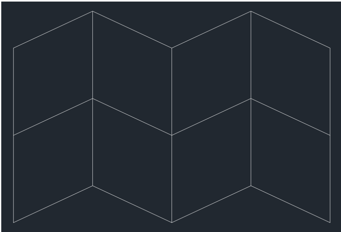
Fig. 14. A computer-aided design (CAD) of a Miura origami (2-unit cells) designed in AutoCAD.
