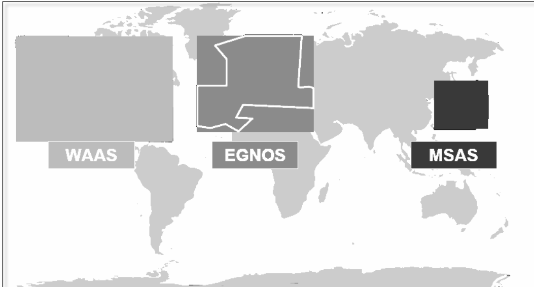
Figure 12. Foot print of Global Deferential corrections services of GNSS: U.S. (WAAS), E. U. (EGNOS), and the Japanese (MSAS).
