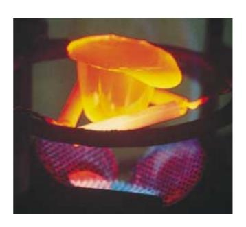
The ignited sample and flux are transferred into a non-wetting platinum alloy crucible and the contents are thoroughly mixed with a chemically inert rod. The uncovered crucible is placed in a muffle furnace or over a gas burner at 900°C to 1,150°C and swirled occasionally until the mixture is completely molten and homogeneous. Samples containing high concentrations of alumina and zirconia necessitate heating at 1,200°C.
