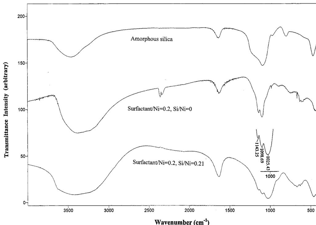
**Figure 11.** Infrared spectra for (a) amorphous silica without nickel oxide, (b) nickel oxide without silicate (surfactant/Ni = 0.2, Si/Ni = 0.), and (c) mesostructured nickel silicate (surfactant/Ni = 0.2, Si/Ni = 0.21).
