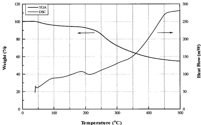
**Figure 9.** TGA and DSC results of mesostructured nickel silicate prepared at surfactant/ $\text{NiSO}_4 = 0.2$  and  $\text{Si}/\text{Ni} = 0.21$ .
