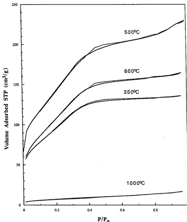
**Figure 8.** The  $\text{N}_2$  adsorption and desorption isotherms of the calcined mesoporous nickel silicate prepared at surfactant/ $\text{NiSO}_4 = 0.2$  and  $\text{Si/Ni} = 0.21$  at elevated temperatures.
