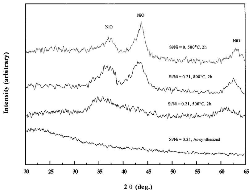
**Figure 7.** XRD patterns of precipitates prepared from  $\text{NiSO}_4$ -CTAB-sodium silicate precursor solutions with surfactant/ $\text{NiSO}_4 = 0.2$  and  $\text{Si/Ni} = 0.21$  at large scattering angles. The XRD patterns for the sample without the addition of sodium silicate is also included for comparison.
