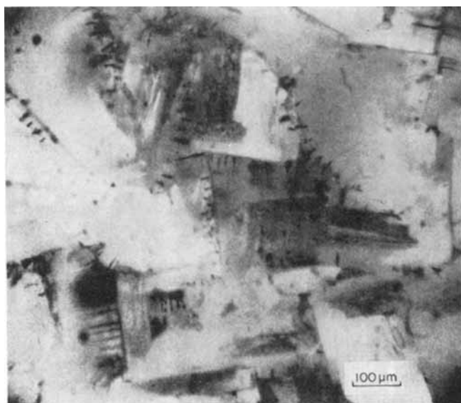
Fig. 2. Microstructure of mullite annealed at 1200°C observed with stereo binocular microscope. Black features are Si particles within the specimen.
