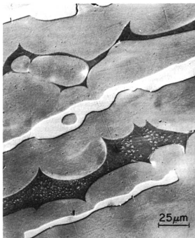
Fig. 4. Microstructure of 71.8 wt%- \text{Al}_2\text{O}_3 -containing silicate melted in sealed Mo crucible at 1953°C for 460 min, cooled to 1753°C in 30 min, annealed at 1753°C for 42,392 min (29.4 days), and quenched from 1753°C to room temperature. Light gray precipitates are alumina completely surrounded by layer of mullite (gray). Dark gray portions between mullite layers are glass containing fine precipitates of mullite formed on quenching.
