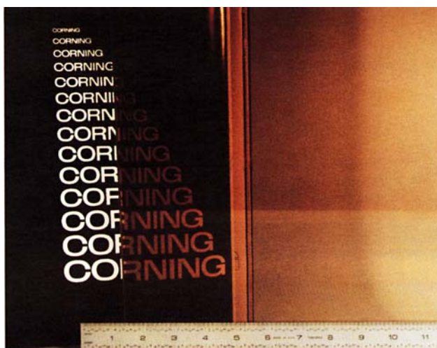
Corning's luminescent window made of \text{Cr}^{3+} -doped mullite glass-ceramic. Low dielectric constant and optical transparency of fine-grained polycrystalline mullite has led to interest in potential applications as a host material as a solid-state laser activator. In highly crystalline glass-ceramic, quantum efficiencies of 30% to 40% have been reported; in glass, quantum efficiencies are less than 1%; in single crystal, efficiencies are close to 100%.
