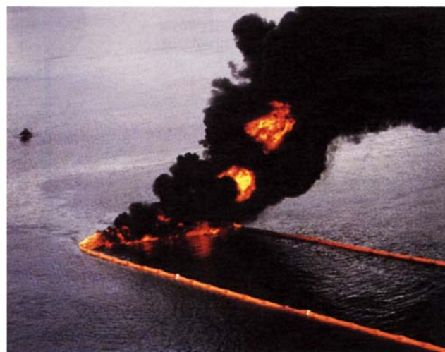
Fig. 8. Mullite fibers are used in thermal and electrical insulation, reinforcement, and high-temperature filtration. Another application is in fire-resistant fabrics to protect booms that are used to collect oil spilled on water. As shown in this figure, using a composite fabric containing NEXTEL 440 ceramic fibers of 3M Co. (3M Fire Boom), the oil may be burned in situ under controlled conditions when retrieval is not possible or practical. High-temperature properties of the fabric allow the boom to maintain an effective oil barrier after exposure to a long, intense oil fire.
