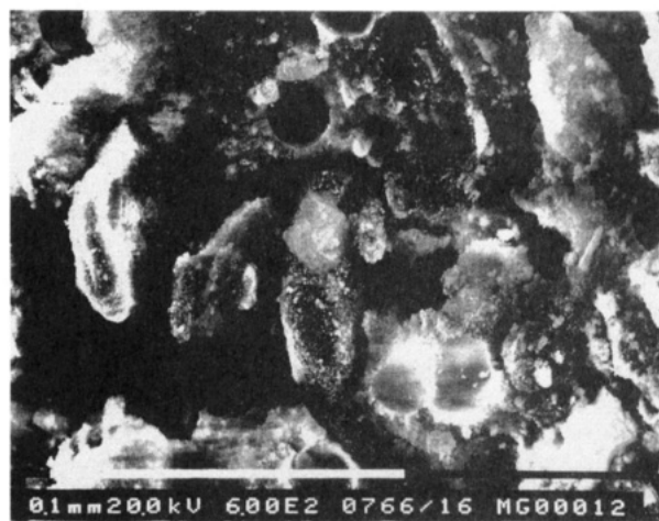
Figure 2. SEM of sintered porous magnetic gel. The circular holes are the locations of the polystyrene beads ( 21.7 \pm 3.2 \mu\text{m} diameter), at a starting volume fraction of 0.015. The voids are the remnants of the polystyrene beads that were thermally removed, while the structure of the gel is maintained.
