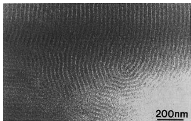
Figure 8. TEM bright-field image of the terrace region of the coordinated barium titanium double alkoxide doped thin film of Kraton. The cylindrical nanodomain spacing of PS (light) is 10 nm, and the barium titanated interdomain spacing (dark) is 23 nm.
