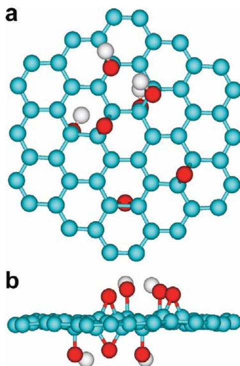
**Figure 1.** Functional groups on graphene. (a) A planar view showing epoxides and hydroxides above and below the graphene plane. Carbon atoms are blue, oxygen atoms are red, and hydrogen atoms are white. (b) Edge-on view of a functionalized graphene sheet with distribution of functionalities above and below the plane. The estimated thickness of a functionalized graphene sheet with functionalities is  $\sim 0.78$  nm.<sup>23</sup>
