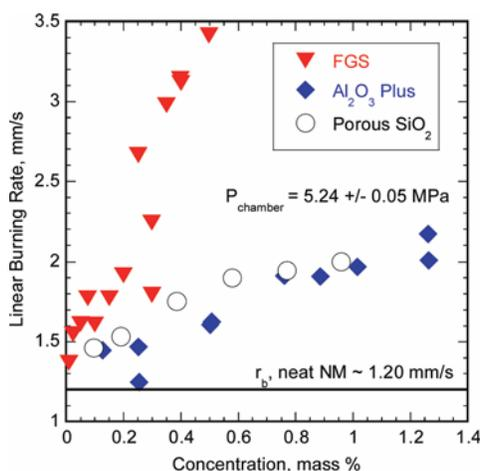
**Figure 5.** Linear burning rate of nitromethane and catalyst support additive mixtures as a function of mass concentration. The burning rate of neat NM is estimated using the experimentally derived correlation from Boyer and Kuo.<sup>34</sup>
