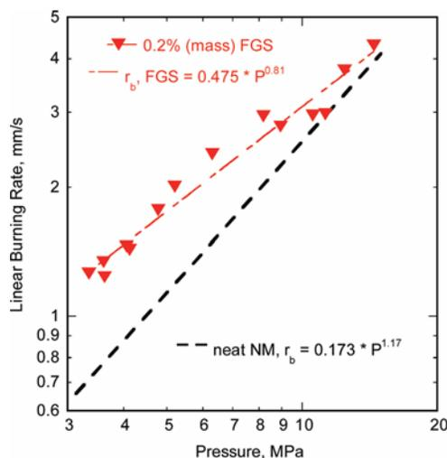
Figure 7. Linear burning rate of nitromethane and FGS additive mixtures as a function of pressure. The burning rate of neat NM is estimated using the experimentally derived correlation from Boyer and Kuo.<sup>34</sup> Burning rate correlations derived for the nitromethane mixtures using a curve fit to the data indicates a greatly reduced pressure exponent (*i.e.*, sensitivity).
