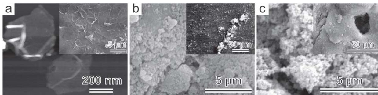
Figure 3. (a) AFM image of single sheet graphene ( $C/O \approx 22$ ). The inset is an SEM image of graphene agglomerates. Also shown are SEM images of (b) Nanoactive Aluminum Oxide Plus and (c) nanoporous silica.
