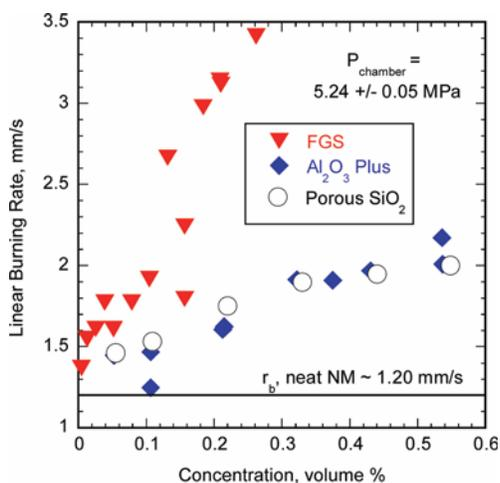
Figure 6. Linear burning rate of nitromethane and catalyst support additive mixtures as a function of volume concentration (density of FGS assumed to be  $2.17 \text{ g/cm}^3$ ). The burning rate of neat NM is estimated using the experimentally derived correlation from Boyer and Kuo.<sup>34</sup>
