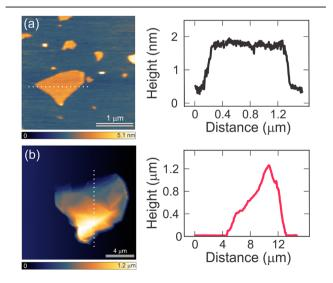
**Figure 9.** AFM images of (a)  $FGS_x$  and (b) FGS-Tz4. The figures on the right of the images show the thickness profile of the particles along white dotted lines.
