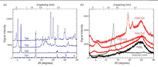
Figure 8. XRD patterns for (a) pure tetrazines after precipitation from solution and (b) the FGS-Tz compounds, GO, and FGS<sub>x</sub>.
