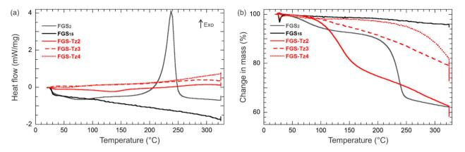
Figure 10. (a) DSC and (b) TG curves for FGS<sub>2</sub>, FGS<sub>15</sub>, and the FGS-Tz compounds. Samples are heated at 5 °C/min under nitrogen to 325 °C and held at that temperature for 1 h to release any bound tetrazine. The TG curves for FGS<sub>2</sub> and FGS<sub>15</sub> are shown for comparison. Residual masses following heat treatment are FGS-Tz2, 58.5% of the original; FGS-Tz3, 73.6%; FGS-Tz4, 72.7%; FGS<sub>2</sub>, 60.2%; and FGS<sub>15</sub>, 95.1%.
