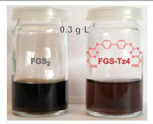
Figure 1. Pictures of 0.3 g·L<sup>-1</sup> suspensions of unmodified FGS<sub>2</sub> (left) and grafted FGS-Tz4 (right) in PC.
