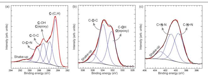
Figure 6. XPS spectra of FGS-Tz4: (a) C(1s), (b) O(1s), and (c) N(1s) core level spectra (red lines) with the results of curve fitting (blue and black lines).
