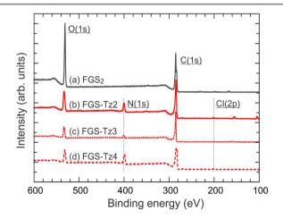
Figure 3. XPS spectra of (a) unmodified FGS<sub>2</sub>, (b) FGS-Tz2, (c) FGS-Tz3, and (d) FGS-Tz4.
