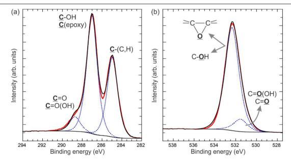
Figure 4. XPS data of unmodified  $FGS_2$ : (a) C(1s) and (b) O(1s) core level spectra (red lines) and curve-fitting results (individual assignments are shown as blue dashed lines; the sum of the curves is shown as a black line).
