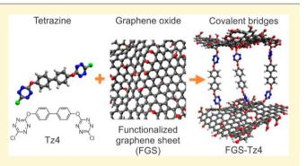
demonstrate that the separation distance between sheets can be maintained while designing new graphene-based materials, including chemically bound, redox structures.
