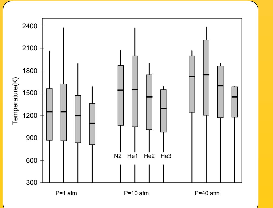
Sensitivity for (R1),  $\text{H} + \text{O}_2 = \text{OH} + \text{O}$ , in  $\text{H}_2$  kinetic model for different diluents at equivalence ratio 2.0.  $\text{N}_2/\text{O}_2 = 1/3.76$ ,  $\text{He}1/\text{O}_2/\text{He} = 1/3.76$ ,  $\text{He}2/\text{O}_2/\text{He} = 1/7.52$ ,  $\text{He}3/\text{O}_2/\text{He} = 1/11.28$ .
