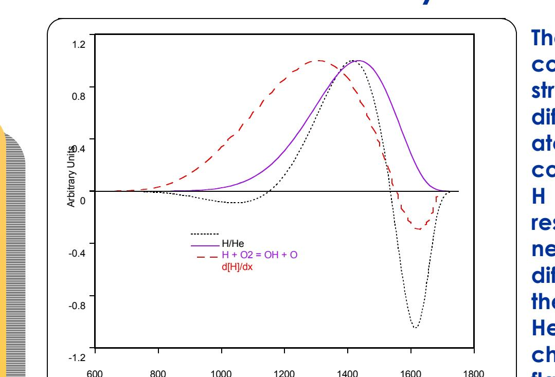
Sensitivity coefficient for  $\text{H}/\text{He}$  binary diffusion coefficient (dotted line), reaction rate of (R1),  $\text{H} + \text{O}_2 = \text{OH} + \text{O}$ , (solid line) and  $\text{H}$  concentration gradient (dashed line) for  $\text{H}_2/\text{He}/\text{O}_2$  ( $\text{He}/\text{O}_2 = 23/2$ ) flame at equivalence ratio 1.5 and 20 atm pressure. All presented quantities are normalized with respect to the maximum values.
