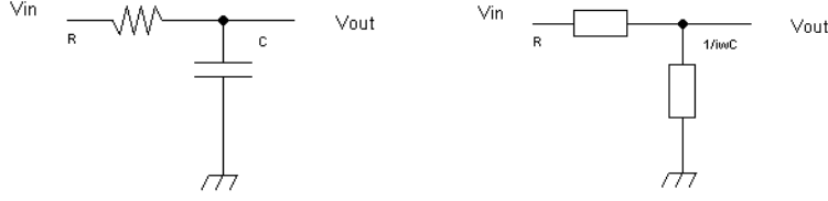
Figure 1: Left: An RC filter. Right: The RC filter in the frequency domain.
