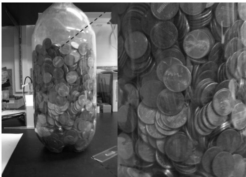
Figure 6. Typical configuration of pennies tossed “randomly” in a container (courtesy of Matt Sullivan). The central region has a packing fraction of 0.574 \pm 0.005 .
