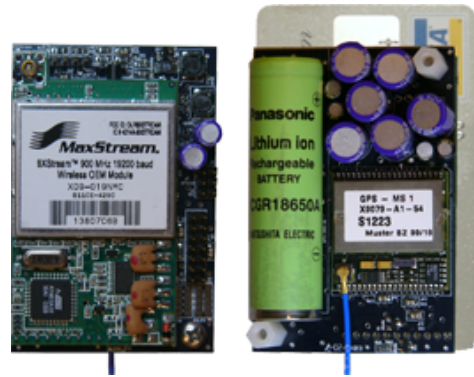
Figure 4: Photo of a ZebraNet node (2"x3"x1.25"). The left card includes the radio and the right card includes the GPS chip and the battery. A credit card is included in the picture for scale.
