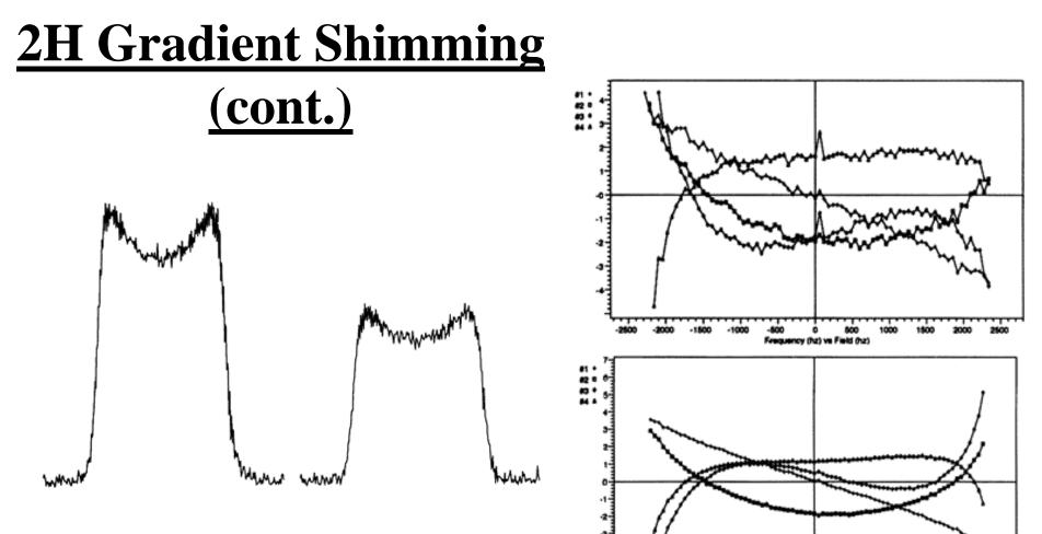
Profiles obtained with at delay set to less than T1 showing "saw tooth" noise.
