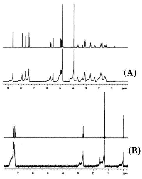
Two panels showing before and after spectra from 2H gradient shimming.
