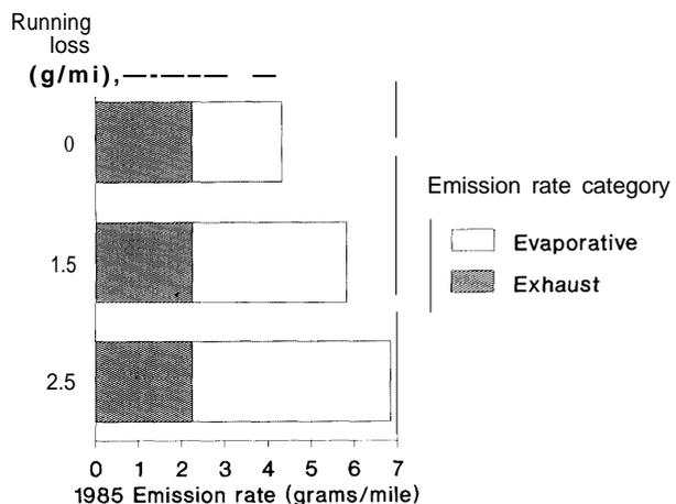
**Exhaust** emission rates do not include the effects of current motor vehicle inspection and maintenance (I/M) programs. We estimate that current I/M programs reduce exhaust emissions by about 12 percent. Estimates of exhaust emission rates assume average vehicle speeds of 28 miles per hour. Emission rates for vehicles in California will be lower since the State maintains a summertime gasoline volatility limit of 9.0 pounds per square inch.
