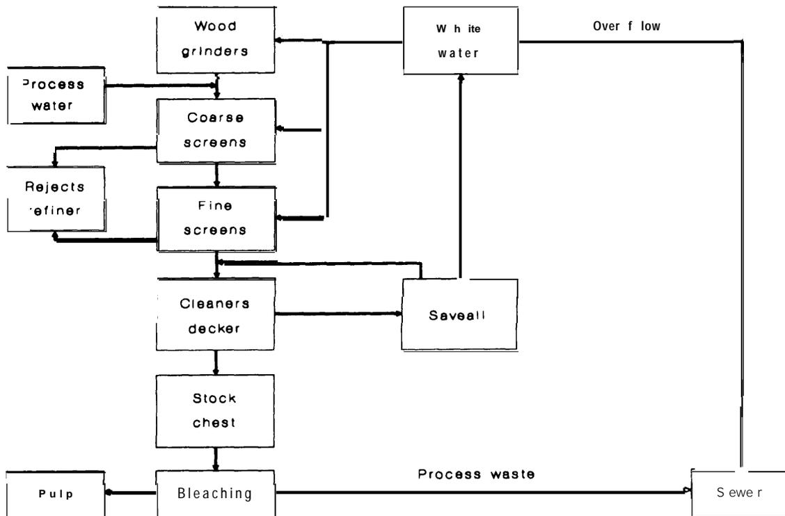
Refiner mechanical pulping (RMP) uses chips in lieu of roundwood and produces paper with higher strength than conventional groundwood because of less damage to the fibers in the pulping process. The chips are passed through a refiner that has fixed and rotating disks operating under a stream of water. A wider range of species, including hardwoods, can be processed by the refiner pulping process. Sawdust and other saw mill wastes can also be used (figure 2-3).
