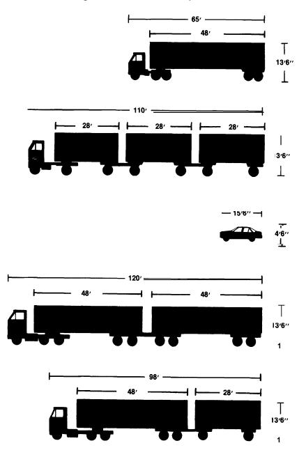
Figure 3-2—Vehicle Size Comparison
