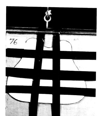
Figure C-3-Mounting Fixtures for Ballistic Tests of Body Armor
