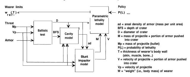
Figure E-9-Alternative Procedure for Estimating Probability of Blunt-Trauma Lethality From Backface Signature and Parametric Lethality Model
