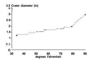
Specifying that backing temperature be measured at several depths and locations and that the drop test be performed both before and after (and perhaps during) ballistic testing would insure that backing temperature is controlled to the current standard, and reducing the allowed temperature range further (e.g., to68to72'F) would further improve control of test conditions and possibly the reproducibility of test results.
