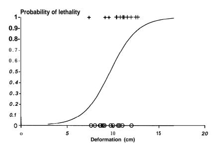
Figure E-5—Lethality Versus Prediction Based on Deformation
