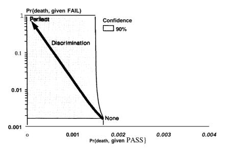
Figure D-3-Confidence Regions for the Probability of Death, Given the BFS Test is Passed, versus the Probability of Death, Given the BFS Test is Failed
