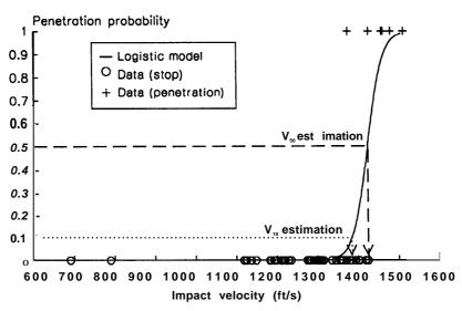
Figure E-2—Estimates of V<sub>50</sub> and V<sub>10</sub> Obtained by Logistic Regression
