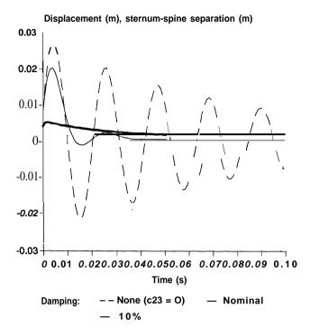
Note that the response is overdamped-i.e., the sternum-spine separation does not oscillate. Also shown are the responses predicted if the damping parameter  $c_n$  were O percent and 10 percent of the nominal value. There is oscillation at about 50 Hz (cydes per second) in both cases, although 10 percent of nominal damping is apparently near critical damping, at which oscillation does not occur.
