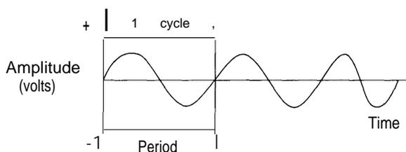
Each cycle of a pure radio wave is identical to every other cycle.
