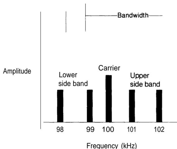
NOTE: This figure represents a 100-kHz carrier wave modulated by 1- and 2-kHz frequencies.
