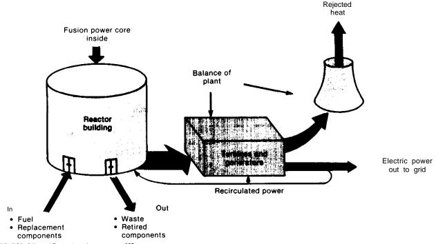
Figure 1=4.—Systems in a Fusion Electric Generating Station
