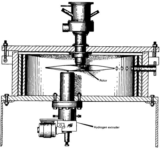
Figure 4-13.—Centrifugal Pellet Injection
