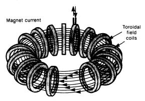
Toroidal field-due to external magnets
