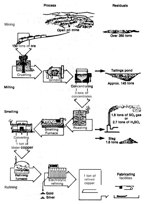
Figure 1.1 —Principal Stages of the Copper Production Process
