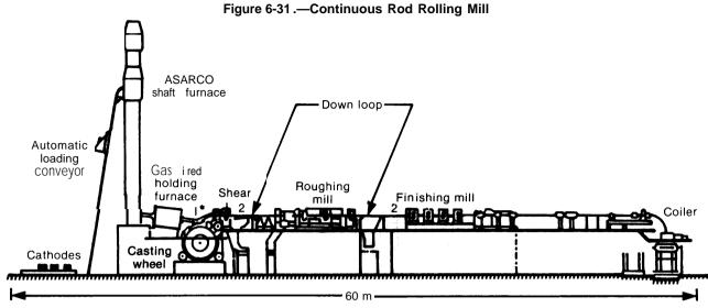
\*NOTE The numbers refer to sensor positions for automatic control
