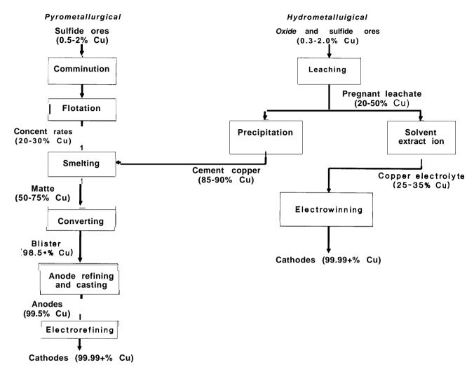
Figure 6-1.-Flow Sheets for Copper Production
