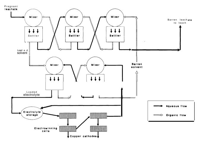
Figure 6-29.-Flowsheet for Solvent Extraction
