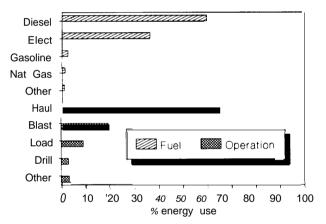
Underground mines use electricity for generating compressed air, pumping, lighting, 'ventilation, and hauling miners and materials. They also use diesel fuel for surface hauling of ore to the mill. Approximately 155 pounds of explosives are used for every short ton of copper produced in underground mines. <sup>5</sup>
