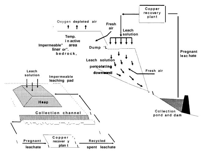
Figure 6-13.-Heap and Dump Leaching
