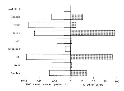
Figure 8-6.-Sulfur Dioxide Control
