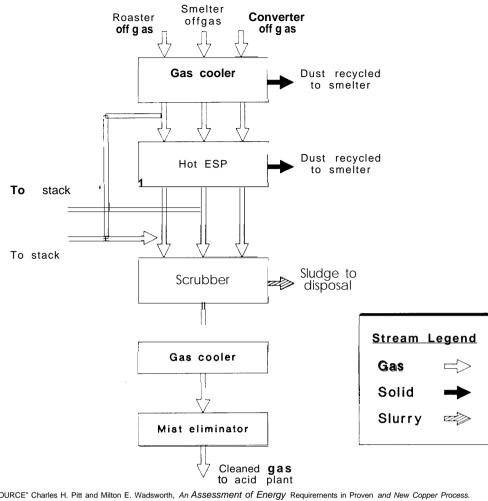
Figure 8-2.-Gas Cleaning in Copper Smelting
