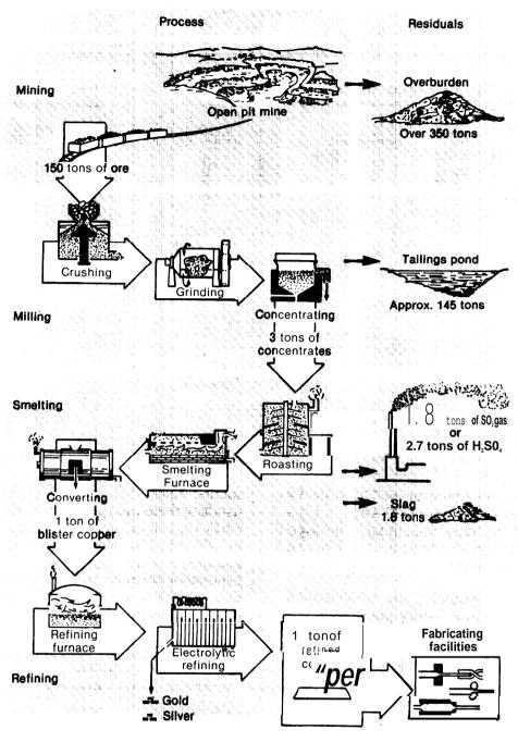
Figure 9-2.— Principal Stages of the Copper Production Process
