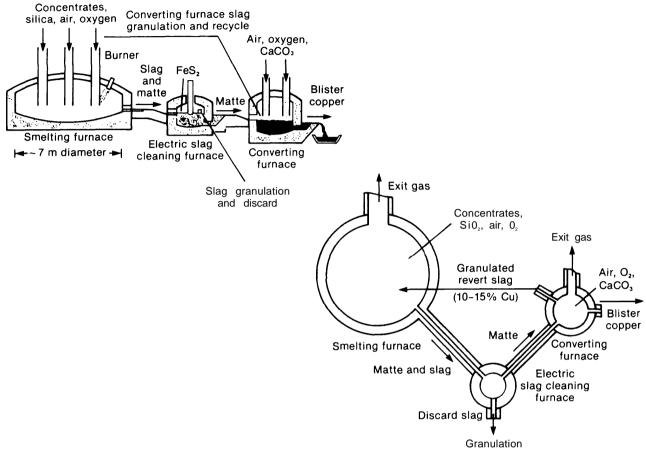
Figure 6-27.—Mitsubishi Continuous Smelting System
