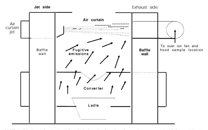
Figure 8-4.-Air Curtain Control System
