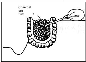
The Egyptian copper smelting furnace was filled with a mixture of copper ore, charcoal and iron ore to act as a flux. It was blown for several hours by foot or hand bellows
