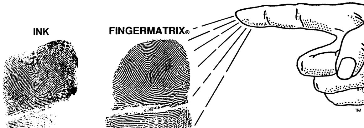
A proprietary electro-optical system scans and digitizes live fingerprints, eliminating inking and rolling. Ten-print fingerprint cards are generated for standard law enforcement use.
