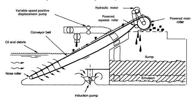
Figure 34-Schematic Drawing of the Navy's Class V Oil Skimmer
