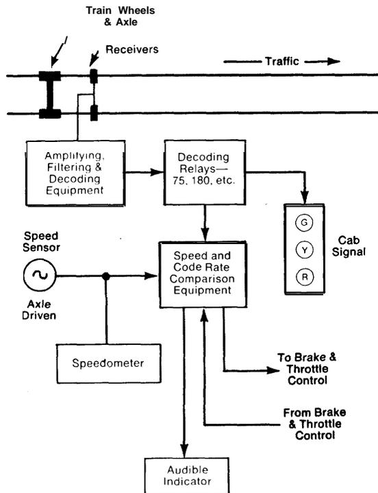
FIGURE 7.—Cab Signal System With Automatic Overspeed Protection
