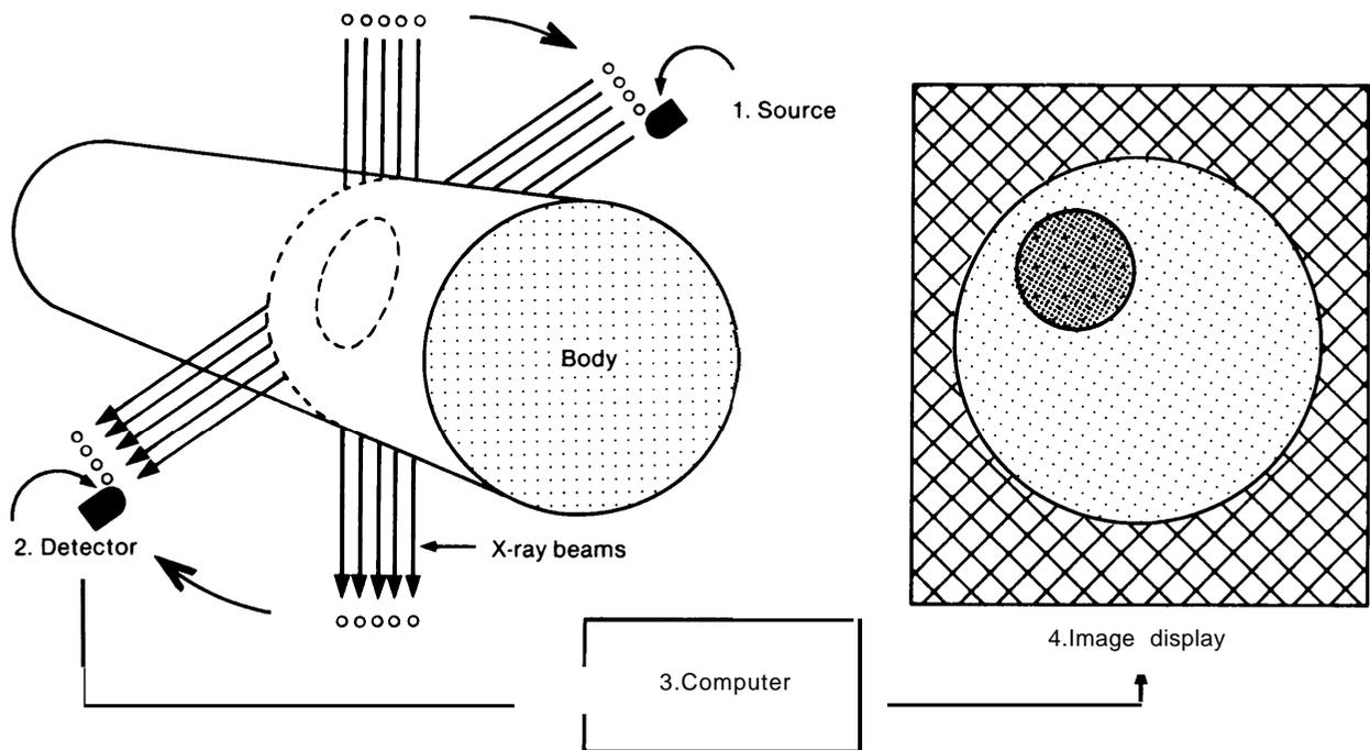
The source and detector are mounted on a single frame and move around the body together in a large number of small steps. X-rays emitted by the source pass through the body and are collected by the detector. Information from the detector is fed into a computer, which reconstructs and displays an image of a cross section of the body.
