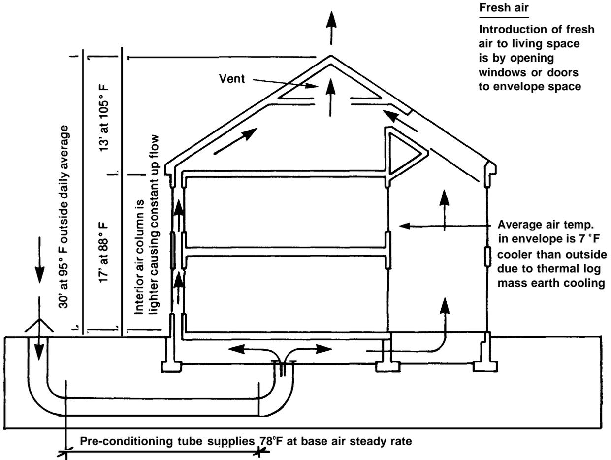
about 12 inches This gap is connected to a basement crawl space and the attic plenums, which in turn are open to the floor and ceiling of an attached greenhouse or solarium. As a result, air can pass in a large loop around the inner structure. Both the inner and outer walls of the double envelope are insulated.
