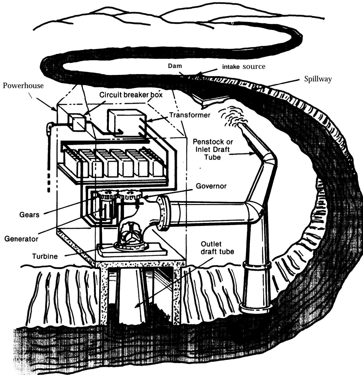
SOURCE: Adapted from: Independent Power Developers' brochure "Hydroelectric Power". Adapted by: National Center for Appropriate Technology in Micro-Hydro Power (U.S. DOE).
