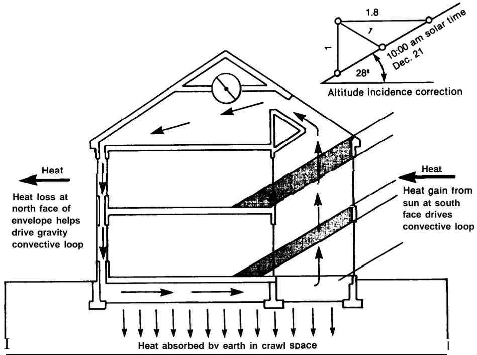
Figure 11.—Thermal Envelope “House, Heat” Loss Cycle
