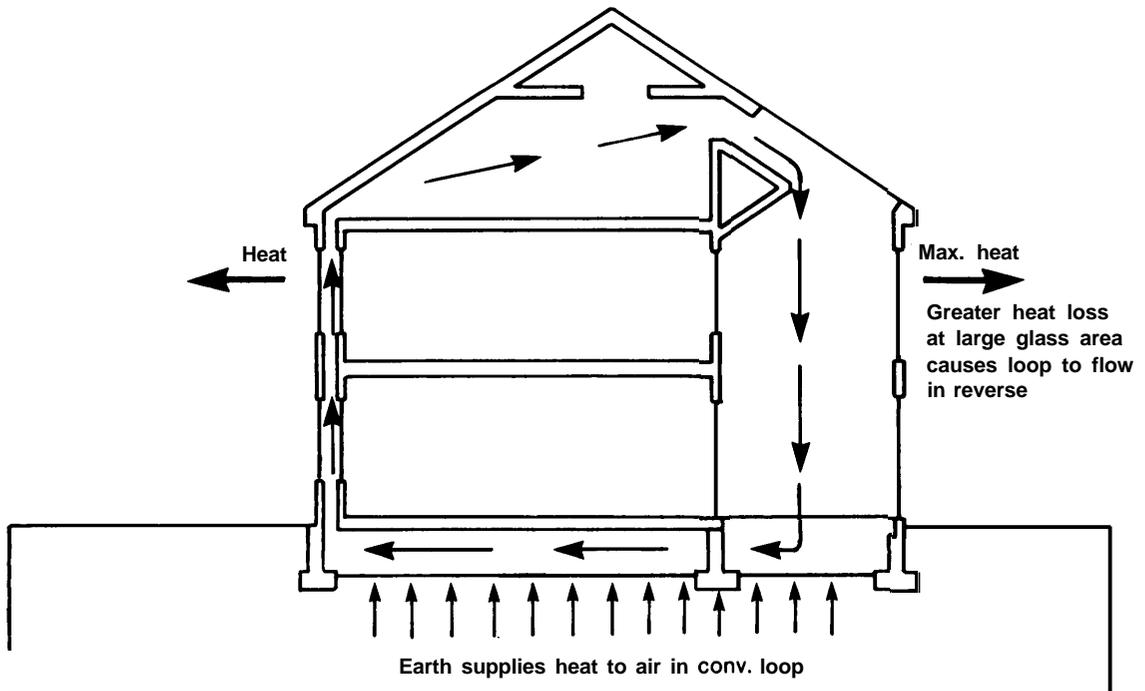
Figure 12.—Thermal Envelope House, Ventilation and Cooling Cycle
