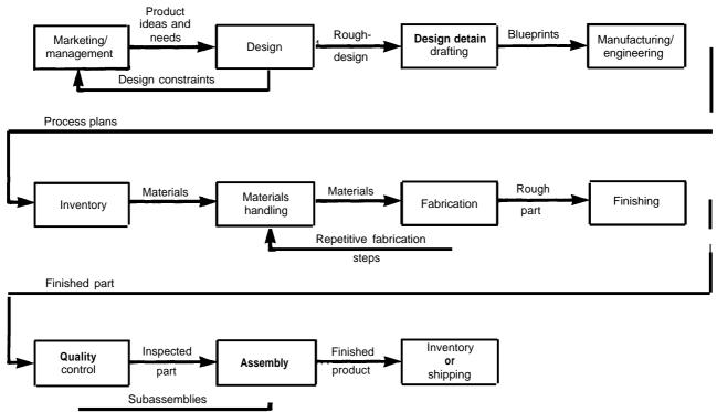
Figure 3.—Steps in the Manufacturing Process (Simplified)
