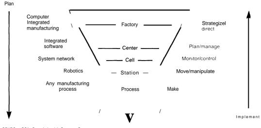
Figure 9.— Programmable Automation Factory Hierarchy (Simplified)
