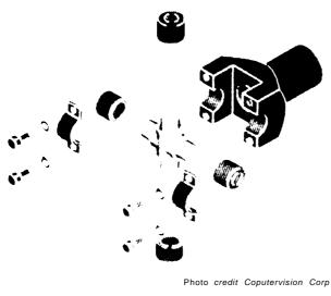
An exploded view of a part assembly from a CAD system with solid modeling capabilities
