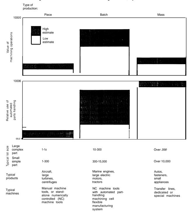
Figure 1 .-- Characteristics of Metalworking Production, By Lot Size
