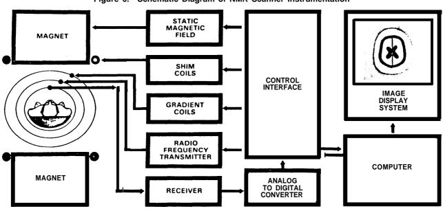
Figure 6.—Schematic Diagram of NMR Scanner Instrumentation
