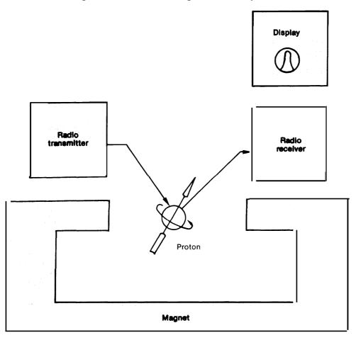
Figure A-2.—Schematic Diagram of NMR System
