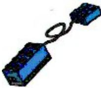
Light Sensor - Connect the light sensor to port 2 on the RCX. Press the VIEW button on the RCX several times. Notice the arrow that moves around the RCX screen. Keep pressing the view button until the arrow points at port 2. Notice the number that is on the screen. This is the light level that the sensor is picking up on a scale of one to one hundred.
