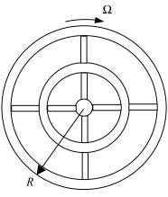
$$\vec{L} = \vec{I} \cdot \vec{\Omega} = \left(\frac{mR^2}{4}\Omega \sin \Omega t, \frac{mR^2}{4}\Omega \cos \Omega t, \frac{mR^2}{2}\Omega\right), |L| = \Omega \frac{mR^2}{4}\sqrt{2^2 + 1} = \Omega \frac{mR^2\sqrt{5}}{4},$$
