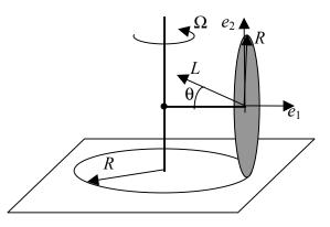
The components of the angular velocity are the same in the lab and rotating frame. Therefore, in the frame of the disk there is a component  $\Omega$  along the axis of the disk and  $\Omega$  along the vertical axis in the plane of the disk:
