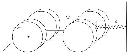
a) Assuming that the wheels of the car roll without slipping on the floor, calculate the frequency of small oscillations of the car
