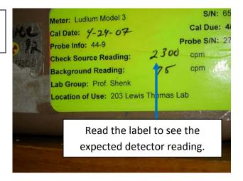
2<sup>nd</sup> step: Turn the knob to the X1 scale (so that the meter reading doesn't go offscale).
