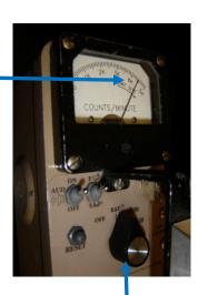
1<sup>st</sup> step: Turn the knob to the 'Bat' position.
