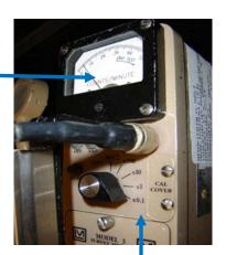
The purpose of the background check is to make sure that the detector is not contaminated or that there are no unusual radiation readings before you begin your survey.
