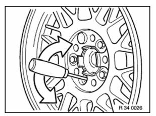
Twist adjusting screw with a screwdriver until it is no longer possible to rotate wheel.
