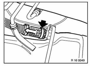
Loosen the ventilation line at the upper side of the fuel tank on the right.
