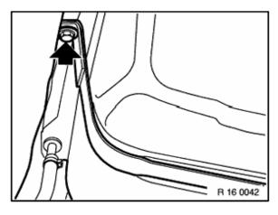
Unscrew and remove front straps.
