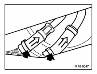
Slightly lower the fuel tank and tilt it forward until the lines can reach the upper side of the fuel tank.
