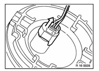
Remove the connection from the sensor for the fuel level gauge on the left.
