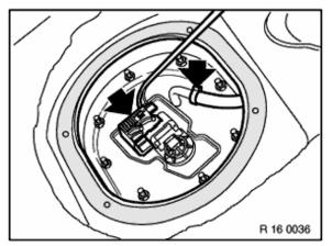
Disconnect the fuel pipe with special tool 13 3 010 and open the hose clamp.
