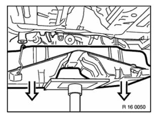
Lower the fuel tank and remove downwards.
