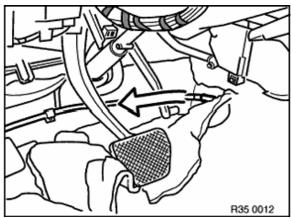
Withdraw Bowden cable from guide tube.
