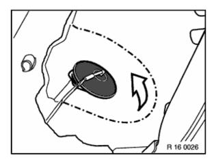
Cut insulating mat along perforated line and fold open.
