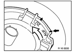
Turn the bayonet lock to the left until the arrow "Open" points to the arrow on the fuel tank.
