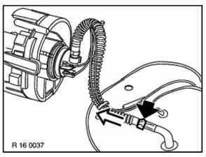
Unfasten hose clip, pull spiral hose off carefully, taking care not to damage the connection.
