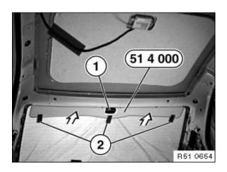
Lift out finisher and disconnect connector.
