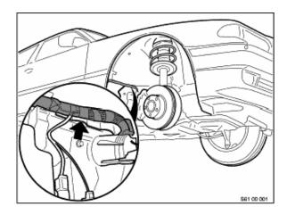
The wiring harness can be damaged by the metal panel (arrow) in the front-right wheel housing
