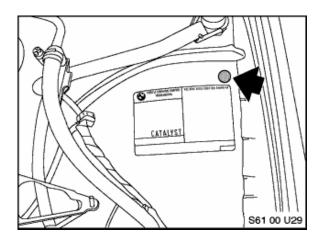
On a customer complaint basis only, where electrical faults have occurred, check for a red mark next to the vehicle emission label (right side of engine compartment).
