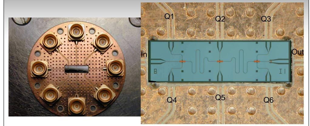
Sample box with 8 x 20 GHz connections
