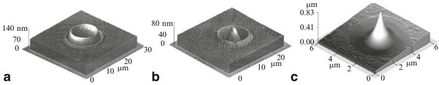
**Fig. 4.2** AFM images of the surface deformations recorded on Ni-P hard-disk substrate at (a) high energy and (b) intermediate energy [38] and (c) 0.8  $\mu\text{m}$  nanotips formed on Si SOI [39]
