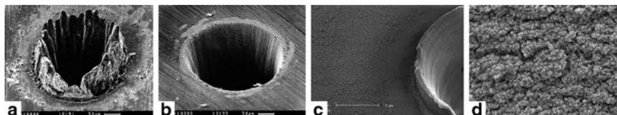
**Fig. 4.3** Laser ablation of holes drilled in a 100  $\mu\text{m}$  thick steel foil with (a) 200 fs, 120  $\mu\text{J}$ ,  $F = 0.5\text{J}/\text{cm}^2$  laser pulses at 780 nm; and (b) 3.3 ns, 1 mJ, and  $F = 4.2\text{J}/\text{cm}^2$  laser pulses at 780 nm [28]. (c) Excimer laser ablation (300 pulses at 193-nm) of zirconium silicate (d) producing vapor-condensed aggregates of nanoparticles in the surrounding regions [47]
