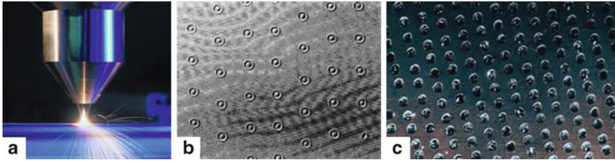
**Fig. 4.4** (a) Laser surface cladding (MTU Maintenance). (b) Micrograph of laser-textured bumps on a super-smooth disk as observed in a phase-contrast microscope [51]. (c) Laser surface texturing of micro-dimples for enhanced tribology [52]
