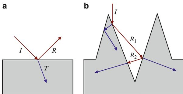
**Fig. 4.6** (a) Light specularly reflecting from a flat surface. (b) Multiple reflections from protruding structures enhance coupling into the material, and refraction causes the light to propagate at oblique angles, increasing the optical path length
