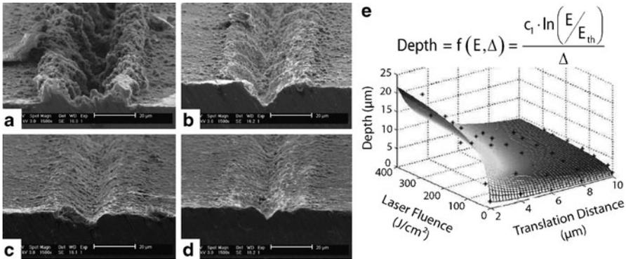
**Fig. 4.11** Cross-sectional SEM images (scale bars are 20 μm) of the laser-machined (56 J/cm<sup>2</sup>) surfaces shows decreasing size and slope of groove walls with increasing translation distance: (a) 2 μm, (b) 4 μm, (c) 6 μm, and (d) 8 μm. (e) Groove depth measurement as a function of translation distance and laser fluence [129]
