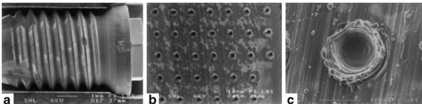
**Fig. 4.10** (a) SEM image of a dental implant that was laser micro-patterned using a kinoform with (b) a regular array of dimples patterned directly onto its threads. (c) A close up of one of the  $10\ \mu\text{m}$  pits showing remnant of material resolidified on the rim and ejected into the surrounding region [128]
