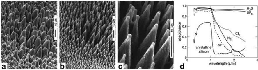
**Fig. 4.8** SEM images of the surface microstructuring of Si(100) by 500 laser pulses of a 200 mm diameter, nearly Gaussian beam (100-fs, 800 nm,  $10 \text{ kJ/m}^2$ ) (a) processed in vacuum and (b,c) in a 500 Torr atmosphere of  $\text{SF}_6$ . Images viewed at an angle of  $45^\circ$  from the surface normal [94]. (d) Absorbance of femtosecond laser microstructured silicon in a variety of gases [95]
