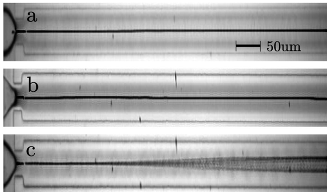
FIG. 2. Plot (dark lines) of the detected center of mass of all bubbles during a flow experiment. (a) For Newtonian solutions, with or without surfactant, bubbles remain in the center of the channel. (b) In a 0.5 wt% 10^6 MW PEO solution without surfactant, bubbles have a similar centered trajectory. No significant deviations from this centered path are observed over the 4 cm length of the device for either (a) or (b). (c) With 0.1 wt % Tween 20 in a solution otherwise identical to (b), bubbles drift from the center to the wall. For sufficiently separated bubbles, motion to either wall is equally probable. All images show an area that is 125 \mu\text{m} \times 3000 \mu\text{m} .
