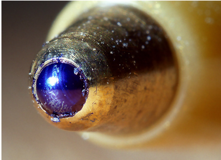
Figure 2: A close-up photo of the ball bearing at the heart of a ballpoint pen. Note the thin film of ink on the ball and the amount of buildup around the edge of the socket. From Wikimedia Commons.
