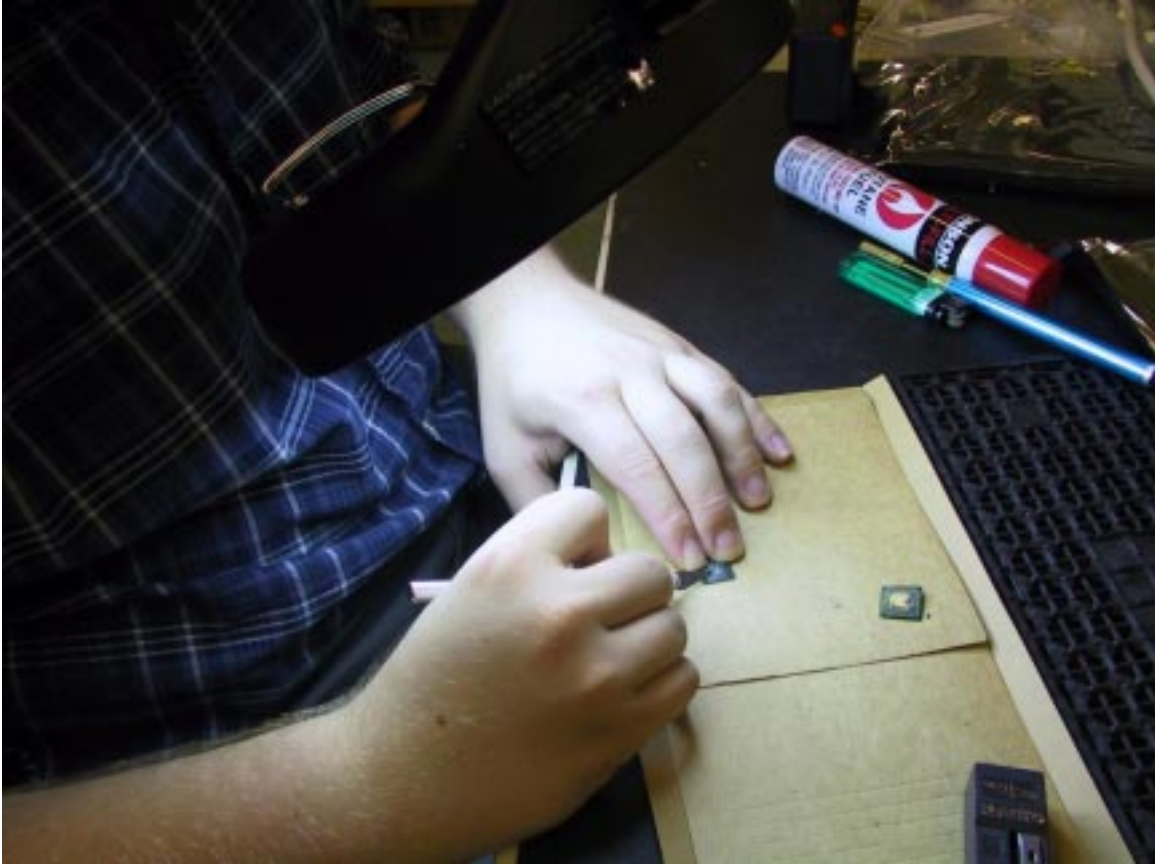
Figure A-6: Removing the FR4 from the Back Side of the Die
