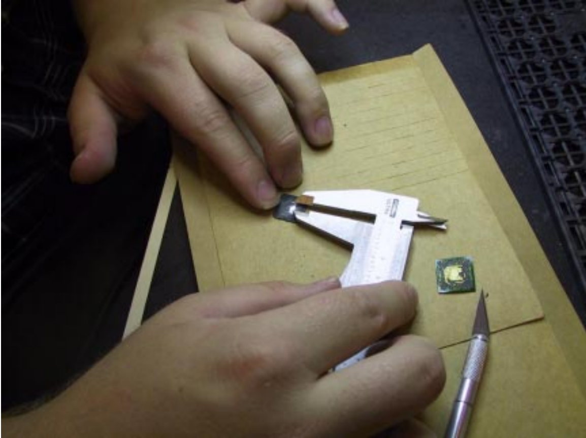
Figure A-7: Measuring the Die Size with Calipers
